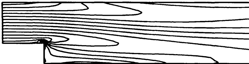
Figure 12. Vorticity contours up to 10 step heights behind backward step, Re = 100 ( \omega = -2.4, -2.1, -1.8, -1.5, -1.2, -0.9, -0.6, -0.3, 0, 0.3, 0.6, 0.9, 1.2, 1.5, 1.8 )
